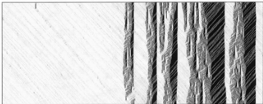
Fig. 15. The (0.11, 0.05, 0.9, 0.9) Traffic Cellular Automaton on 1,000 sites, from 79,600 to 79,999 updates, with density \rho = 0.3 .
